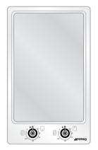
The symbol adjacent to the knobs indicates the cooking zone they control. To switch a zone on, turn the knob to the desired position. Adjustment is continuous, so the appliance functions when set to the intermediate values as well. To switch off a zone, reset the knob to  $\mathbf{0}$ .
