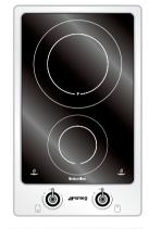
The symbols alongside the knobs indicates the cooking zone they control. To switch a zone on, press the knob and turn it to the desired position. Adjustment is continuous, so the appliance functions when set to the intermediate values as well. To switch off a zone, reset the knob to  $\bf 0$ .
