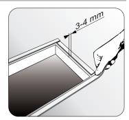
Carry out this operation by supporting the hob on the isolating seal and using screws and clamping brackets to fix the hob to the support structure, in order to obtain the complete flatness.
