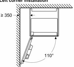
If using the 92° hinge limiter, the min. distance to the wall is only 100  $\,\mathrm{mm}$
