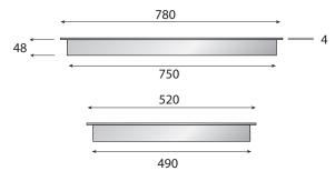
Model: ILD784B Cut out (LxD) : 750 x 490mm – thickness : 48 mm + 4mm glass Size (LxD) : 780 x 520 mm, R=5 Electrical network 220-240 V, 50/60 Hz Total Electrical Consumption: 7.1kW/h
